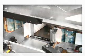
The Vantra IM cartoner/tray packer provides a highly versatile single platform solution designed with a hygienic sheet metal frame and standoff bearing mounts.
