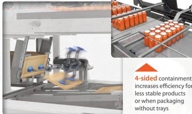
**4-sided** containment increases efficiency for less stable products or when packaging without trays
