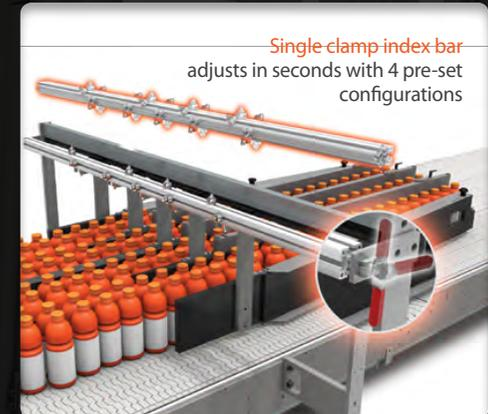
Single clamp index bar adjusts in seconds with 4 pre-set configurations
