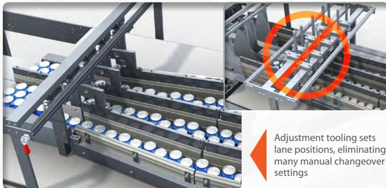
Adjustment tooling sets lane positions, eliminating many manual changeover settings
