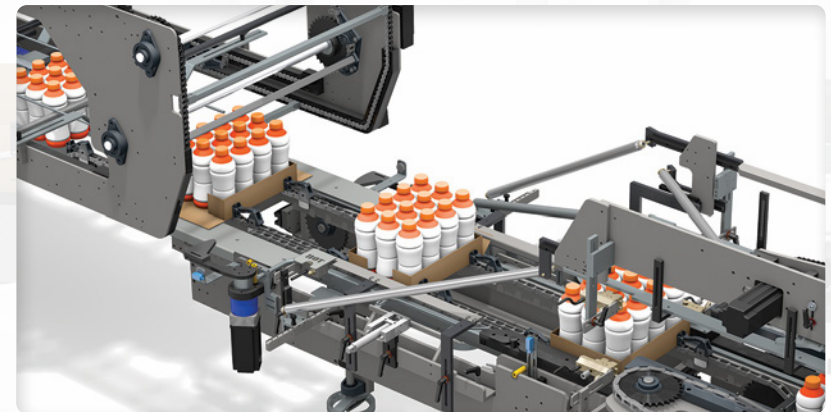
Trays: Conventional end-slotted trays run wide-side leading
