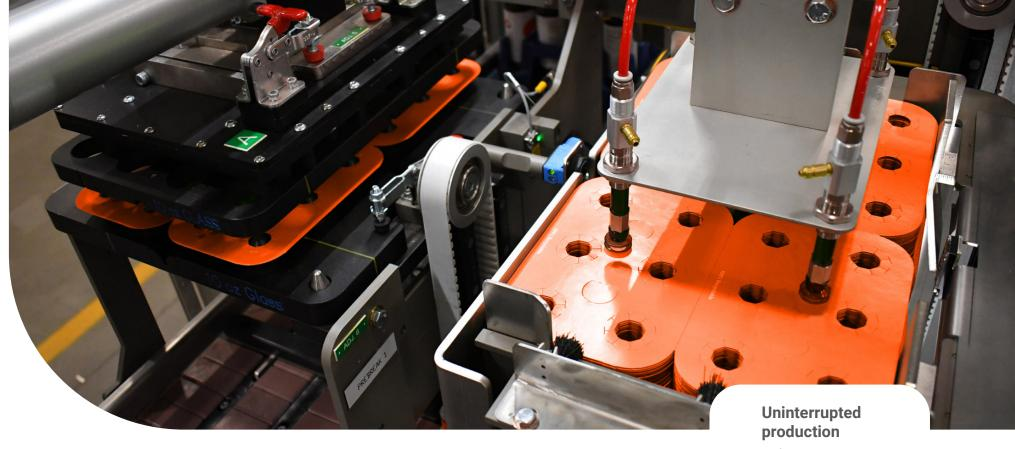
Robotic applicators with Rockwell controls offer low maintenance and easy, tool-less changeovers that maximize uptime
